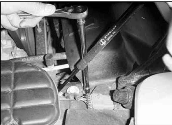
28. Loosen and remove the four bolts that retain the upper radiator cover.
