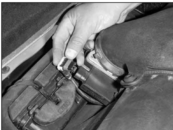
2. Disconnect the mass air sensor electrical connection.
