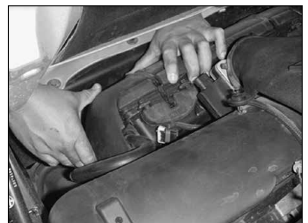
6. Pull the airbox towards the engine to release it from its mounting grommets.
