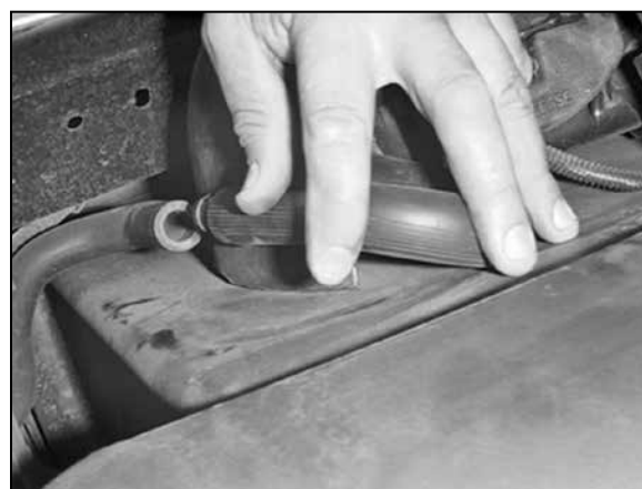
3. Disconnect the air injection vent hose.
