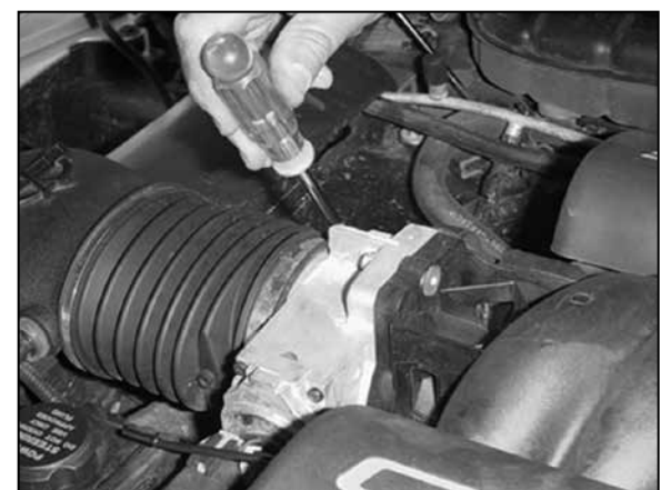
5. Loosen the hose clamp on the intake hose at the throttle body.
