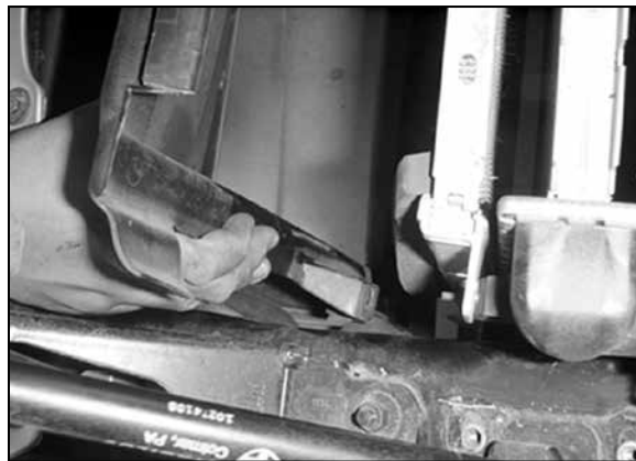
33. Pull firmly to release the radiator cover from its retaining clips.
